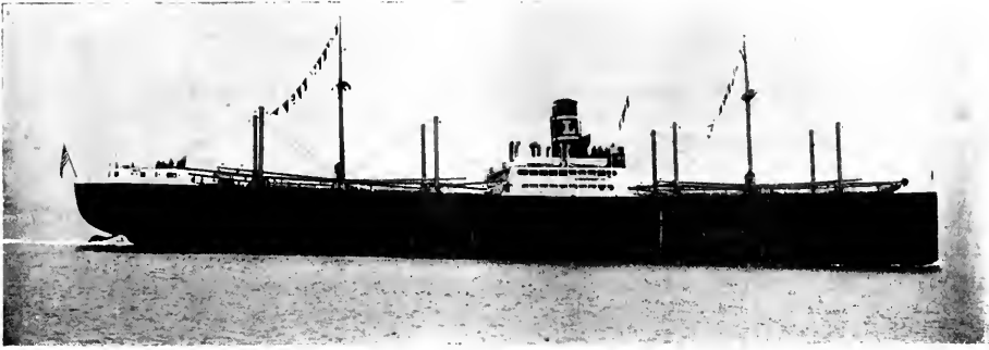
The "Edward Luckenbach," one of the cruiser-sterned steamers of the Luckenbach fleet.
